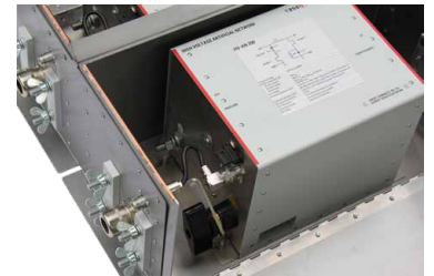
Flexible HV connection
