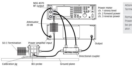
Attenuator: 20 dB, 10 W Termination: 50 Ω 10 W
