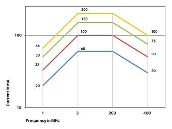
Test level — for ISO 11452-4:2011 Level 1 Test level — for ISO 11452-4:2011 Level 2 Test level — for ISO 11452-4:2011 Level 3 Test level — for ISO 11452-4:2011 Level 4
