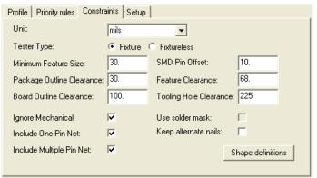
Probe locations may already be defined within the CAD data, but there may be insufficient access for total test coverage. In which case the probe analyzer can be used to consider alternative top and bottom side accessibility options such as through hole pins (THT), connectors, SMD pads, vias or bead probes etc.
