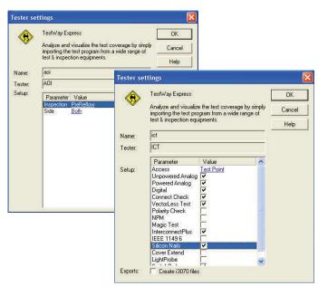
**TestWay Express** handles cross optimization along the test line such as Boundary-Scan or AOI that can be used to minimize the In-Circuit Test or Flying Probe Test.
