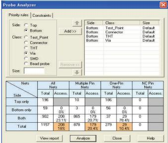
Once the possible probe positions have been analyzed, the nail allocation algorithm selects the best of these opportunities for the nail positioning according to the preferences set by the user.
