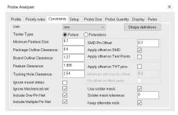
Probe locations may already be defined within the CAD data, but there may be insufficient access for maximum test coverage. In which case the probe analyzer can be used to consider alternative accessibility options, such as through hole pins (*THT*), connectors, SMD pads, vias or bead probes etc.
