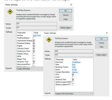
**TestWay Express** handles cross optimization along the test line, such as Boundary-Scan or AOI, that can be used to minimize the cost of In-Circuit Test or Flying Probe Test.
