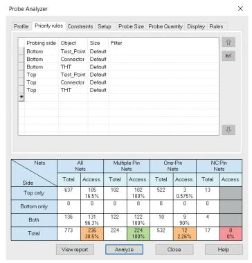
Once the possible probe positions have been analyzed, the nail allocation algorithm selects the best of these opportunities for the nail positioning, according to the preferences set by the user.
