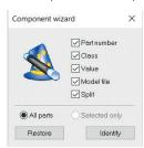
A component wizard is provided to simplify the component modeling, automatically identifying device classes, importing any available models and extracting valuable component information, such as value, tolerance, shape etc, directly from the BOM description.
