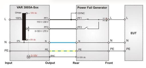
**Voltage interruptions (DIPS)** will cause a reduction of the power supply voltage for a certain period of time, three different test levels are required in IEC/EN 61000-4-11:
