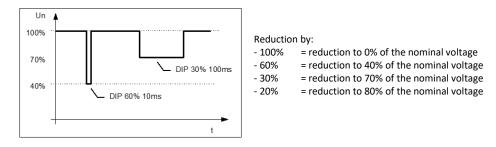
**Additionally** it is possible to drive certain functions of **voltage variations**, which also are required in older versions of the standard IEC 61000-4-11. These functions can easily be programmed within the simulators itself or within the related windows software.
