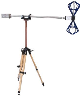
VSQ 3002, assembled for the frequency range 30 to 1000 MHz
