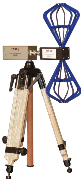
VSQ 3002, alternative setup below 1 GHz: DPA 4000A mounted direct on RSG 3000
