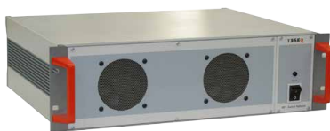
RF Switch network for high power, view to the front panel
