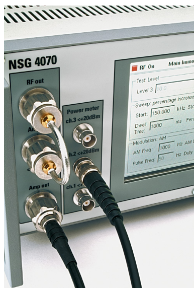
NSG 4070 front panel with RF ports
