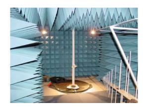
ETS-Lindgren's SpaceSaver™ PC is a semi-anechoic chamber, designed to perform ANSI C63.4/CISPR 16-1-4 and IEC 61000-4-3 pre-compliant radiated immunity measurements. This chamber can also be used for ANSI C63.4 pre-compliant radiated emissions measurement prescans, with limited height scan. Frequency ranges for this chamber are 80 MHz to 40 GHz (radiated immunity) and 30 MHz to 40 GHz (radiated emission).
