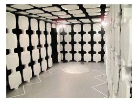
The SpaceSaver™ 26H is an RF-shielded semianechoic chamber providing a multi-purpose environment for radiated immunity and precompliant emission testing. This compact chamber provides an anechoic test environment that supports testing up to 40 GHz with anechoic performance equal to or better than that required for radiated immunity testing per most standards including IEC, pre-compliant emission testing,
