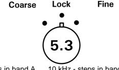
Coarse: 100 Hz - steps in band A 10 kHz - steps in band B Fine: 10 Hz - steps in band A 1 kHz - steps in band B
