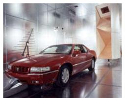
ETS-Lindgren's SMART™ (Statistical Mode Averaging Reverberation Test-Site) Chambers use the latest developments in proven reverberation technology and experienced chamber design and construction, to create a suitable electromagnetic environment (EME) for immunity, emissions and shielding effectiveness testing. Compared with other test methods, SMART chambers offer the advantages of lower cost, higher field-to-input power ratios, and the ability to accept large test systems.
