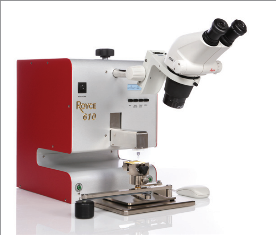
The Royce 610 has an optional strip printer unit that allows you to print out a hard copy of test data. The 610 can also be linked to the centralized database by using the Royce SurePC option.
