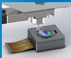
UV dispensing on camera module
