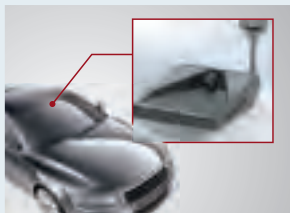
ADAS holder bonded to windshield
