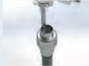
Waterproof sealing of connectors
