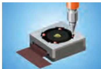
UV dispensing on camera modules
