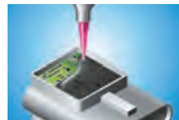
Pressure Sensor Potting
