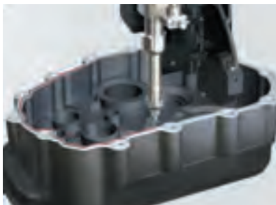
FIPG dispensing on engine parts
