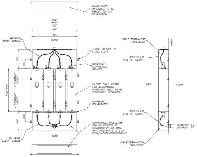
As installations of high current filters can depend largely on where the power cables are situated, a customised installation kit may be required. MPE can work with your specific requirements to develop bespoke termination enclosures, bus-bar piercings and enclosure piercings to suit your installation.
