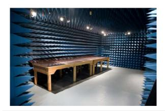
ETS-Lindgren's MIL-STD-461 chamber is designed for testing in accordance with Mil-Std 461E, Mil-Std 461F and Mil-Std-461G. The chamber's shell is constructed with Series 81<sup>TM</sup> modular cell-type shielding panels. Interior end walls, portions of the sidewalls and ceiling are lined in the manner required by MIL-STD-461, using EMC-24PCL absorber.
