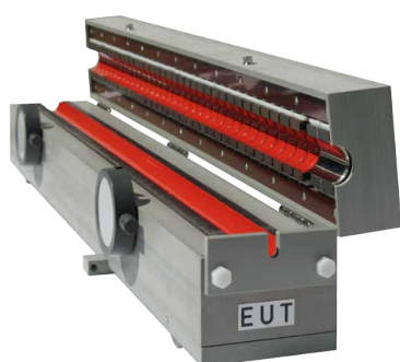
View to the EUT side of the opened MDS 21B
