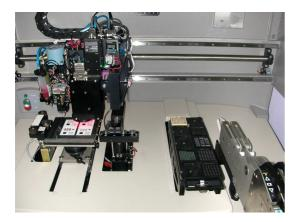
Performs MCM, Hybrid, Flip Chip, Eutectic, Silver Glass die attach applications.
