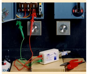
**COMPLIANCE** The PLIP is designed to comply with the CISPR16 requirements for a voltage probe. The design incorporates several features that are in addition to the basic CISPR16 specifications.
