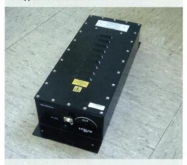
The military specification LISNs are part of a wid range of EMC test equipment available froi Laplace. These Defence Standard LISNs ar characterised by a demanding performance specification extending up to 400MHz.
