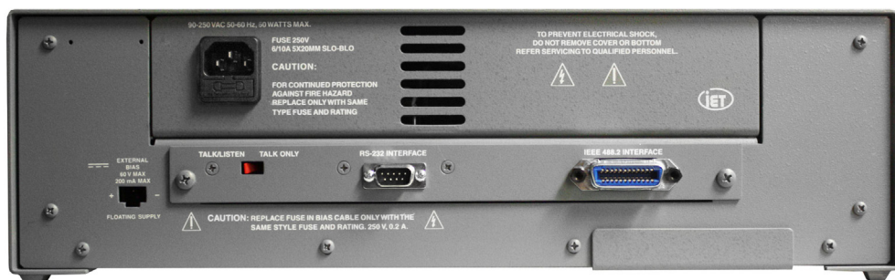
Rear view of 1693 RLC DigiBridge with optional IEEE-488 interface
