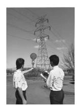
ETS-Lindgren's HI-3604 ELF Survey Meter is a magnetic field probe designed to evaluate both electric and magnetic fields associated with 50/60 Hz power lines, line-powered equipment and appliances. The HI-3604 ELF (extremely low frequency) Survey Meter provides the engineer, industrial hygienist and health and safety professional with a sophisticated piece of surveying equipment for accurate investigation of power frequency environments.
