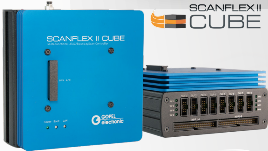
USB/LAN controller for up to eight units under test
