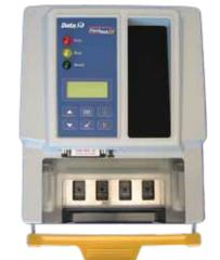
The FlashPAK III features a low profile ergonomic design in a small desktop footprint. This design enables operators to easily run multiple FlashPAK's at the same time increasing production throughput. Lifting the unique socket Actuator Bar starts the programming process. One unit can program up to four devices in parallel.
