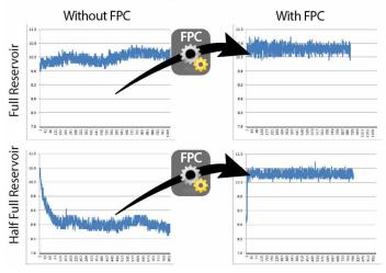
Any fluid fed from a reservoir with constant pressure applied, may flow at varied rates. This is very evident with large reservoirs of thermal grease, gasketing material, or RTVs. When starting to feed fluid from a large, full reservoir into the pump, a certain pressure is required. If that pressure remains constant as reservoir fluid is depleted, the flow rate of the fluid entering the pump will vary, causing a difference in pump output and/or performance.
