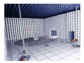
ETS-Lindgren FACT<sup>M</sup>10 Chambers, for Full Compliance testing, offer semi-anechoic radiated emissions (RE) and fully anechoic radiated immunity (RI) compliance test capability for most international EMC compliance regulations. The chamber's small overall size results from the use of brand hybrid absorber and ferrite tile, which require less volumetric space than traditional absorbers. ETS-Lindgren FACT 10
