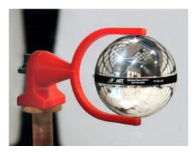
ETS-Lindgren's Universal Spherical Dipole Source (USDS) is an instrument that helps you maintain the integrity of your test environment (chamber or OATS). It does this by allowing you to create a radiated emissions profiles that can be compared with other profiles made on a daily basis. Differences in profiles can indicate changes occurring in the test environment that may affect the accuracy and repeatability of test results.
