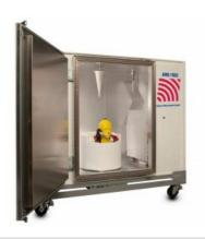
ETS-Lindgren's AMS-7000 Wireless OTA Reverb Test System is designed to perform accurate and repeatable SISO TRP, TIS, Throughput, and MIMO Throughput measurements. The system is based on the company's long-standing line of SMART<sup>™</sup> reverberation chambers and proven EMQuest<sup>™</sup> antenna
