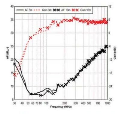
3143B BiConiLog Antenna Beamwidth **Typical Performance**
