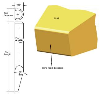
This style of tool has no feed hole and is used on very small pads. Usually manual Bonders are used. The wire is first positioned over the bonding pad area then the wedge is lowered onto the wire to make the bond. This operation can be thermo compression, thermosonic, or ultrasonic type bonding. We have tried to cover most bonding styles in this series for your requirements. If we have not shown a style for your needs please contact the Engineering Department for your custom design.
