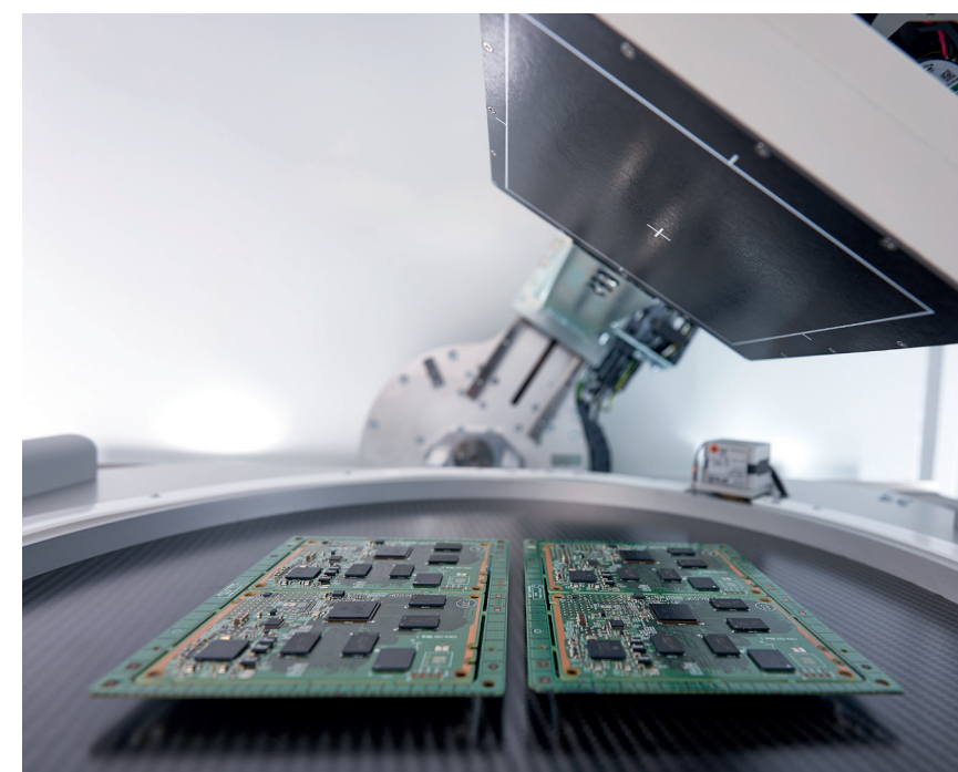
Automated 2D and laminography inspection for maximum productivity.
