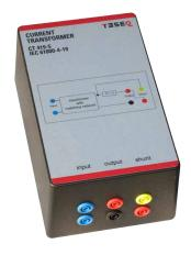
offers with CT 419-5 a transformer with integrated matching network for testing EUTs like electricity meters. The CT 419-5 is fully compliant with the requirements of the standard and provides a simple and reliable method of injecting differential mode current into the equipment under test (EUT).
