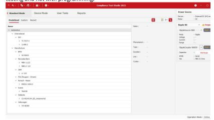
Using the standards library for testing is a convenient way to get started quickly. Select one of the pre-programmed tests, adjust the basic settings and start the test. The library for the Ripple NX covers international automotive standards (e.g. ISO 21498-2 and ISO 7637-4, CTS.Automotive-INTL license required), as well as many OEM standards (e.g. Stellantis, Volkswagen, Mercedes etc., CTS.Automotive-MFC license required).
