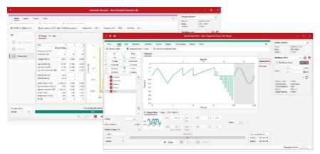
The Device Mode allows to remotely control the device and access to functionality beyond what is required by the standards. It gives full control to both the basic and advanced features.
