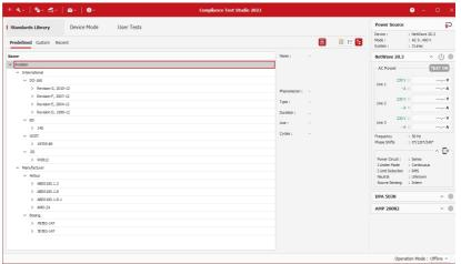
Tests cover voltage variations with a NetWave (swells, dips, frequency changes, unbalance etc.), power analyzer measurements with option NWB (current consumption, power, power factor, inrush current, harmonics emissions etc.) and audio frequency conducted susceptibility with an AMP 200N.
