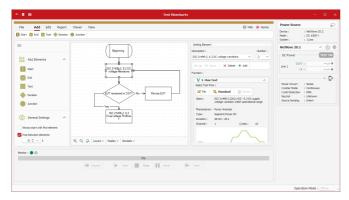
The Waveform Editor allows easy programming of AC and DC voltage variations. Use the pre-programmed waveforms from the Standards Library, customize it to your needs or program a custom waveform based on the available segments (ramps, transitions, distortion, sweeps etc.). The waveform is changed by modifying the segment parameters which are documented in the integrated help.
