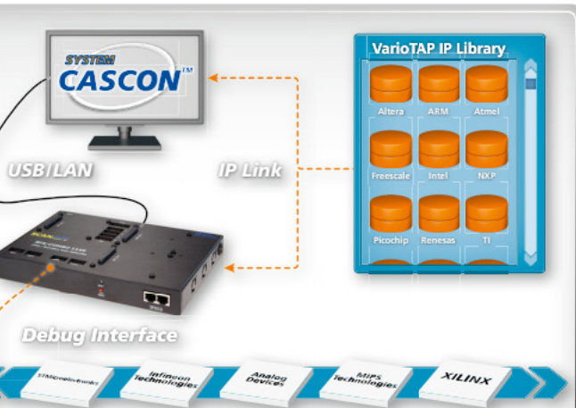
Example of the functional principle of VarioTAP®
