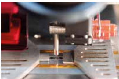
Scrubbing motion or Ultrasonic bonding action
