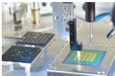
Stamping unit for adhesive application
