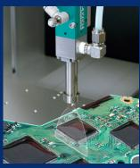
Spot coating by non contact high speed jet.
