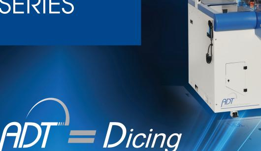
The ADT 7900 series Dicing Saws has two facing spindles that can simultaneously dice wafers or packages at high throughput. ADT 7900 series is a high accuracy system that can dice product at high performances and low cost of operation.
