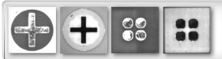
Fiducials detection with visible light and with ultraviolet illumination
