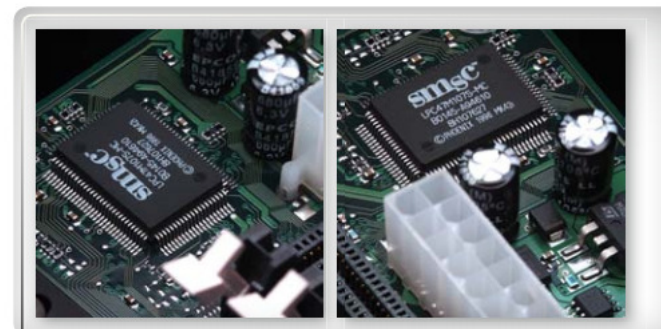
Inspection of hidden fine pitch IC with angled-view Chameleon module
