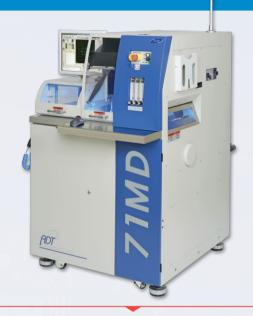
The 71MD dicing system is designed for demanding and tight applications such as PZT. The system is equipped with Height on parts measuring system and it can be provided with large Z clearance. It can also be supplied with a balancing tool to minimize spindle vibration, typical for Ultra-Sound sensors applications.
