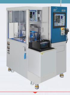
ADT 8030 Dicing system has two facing spindles that can simultaneously dice wafers at high throughput. ADT 8030 is a high accuracy system that can dice product up to 12" in diameter or  $12" \times 12"$  product, at high performances and low cost of operation.
