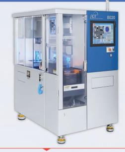
ADT 8020 Dicing system has two facing spindles that can simultaneously dice wafers at high throughput. ADT 8020 is a high accuracy system that can dice product up to 8" in diameter, at high performances and low cost of operation.
