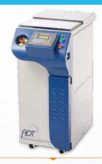
Designed for after-dicing workpiece cleaning and drying. Equipped with a spinning chuck table and a rotating washing/drying arm. The arm can be configured with an atomizing cleaning nozzle or a high pressure nozzle to cope with a wide range of cleanliness requirements.
